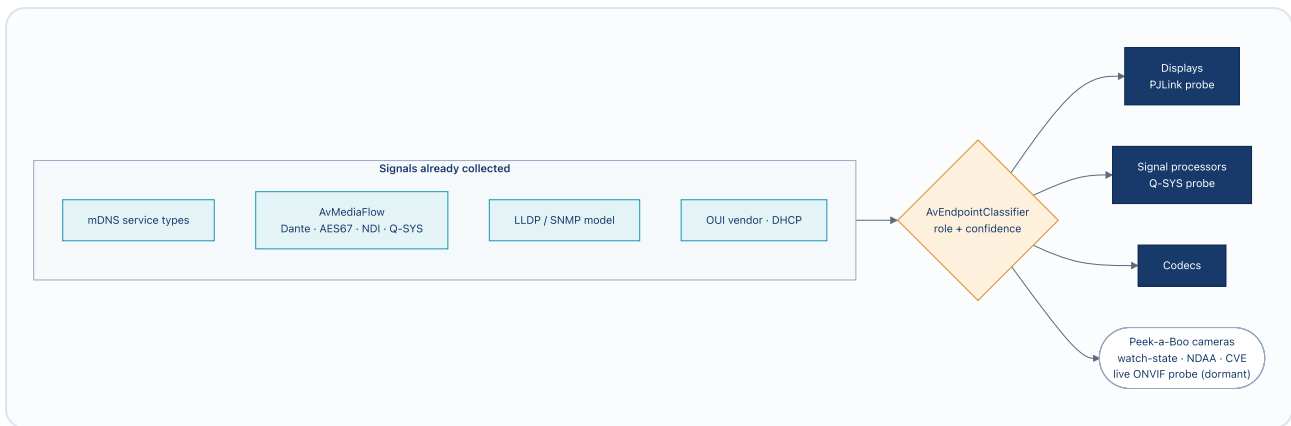
Figure 2. One classifier, many AV modules. The production classifier types every AV device from signals already collected; the per-type modules add a live read. Peek-a-Boo is the experimental camera module on top, with its deeper live-streaming probe dormant until credentials are supplied.
