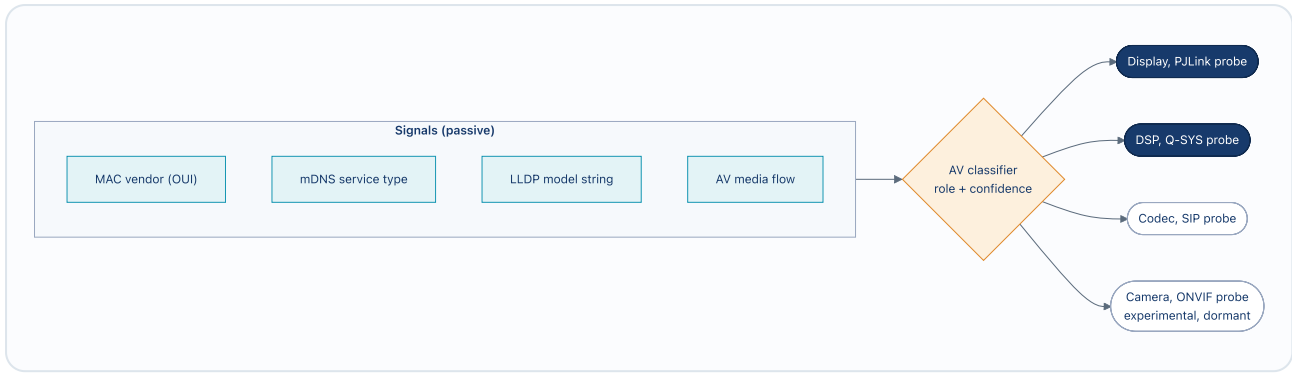
Figure 2. AV vendor to role to probe. The MAC vendor and passive signals classify a device into an AV role with a confidence label; where a standard management protocol exists, a live probe confirms it. The camera (ONVIF) probe is the experimental Peek-a-Boo path and stays dormant until enabled.
