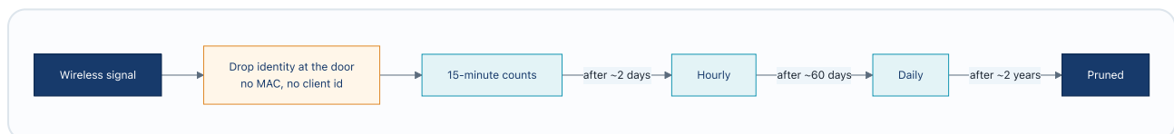
Figure 7. Identity never lands. Any client identifier in an incoming event is hashed with a per-run salt and dropped at ingest; only counts survive, and they age down a retention ladder.
